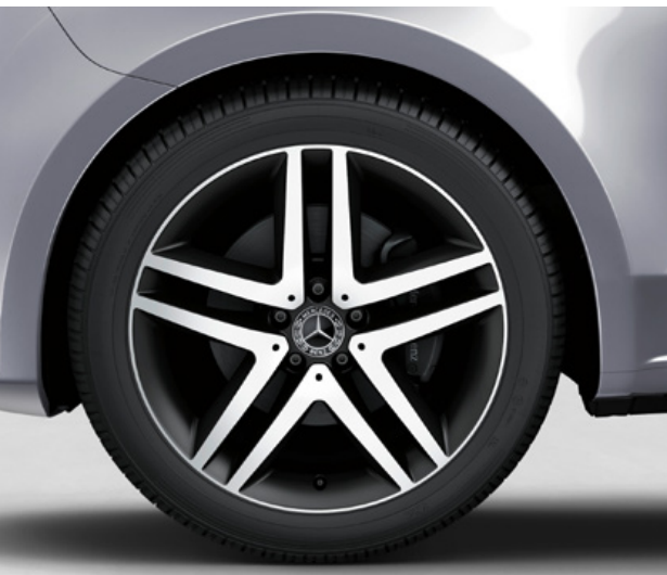
RL3 19" AMG alloy wheels (4) – 5-twin-spoke design painted in black with a high-shine front front: 245/45 tyres; rear: 245/45 tyres
