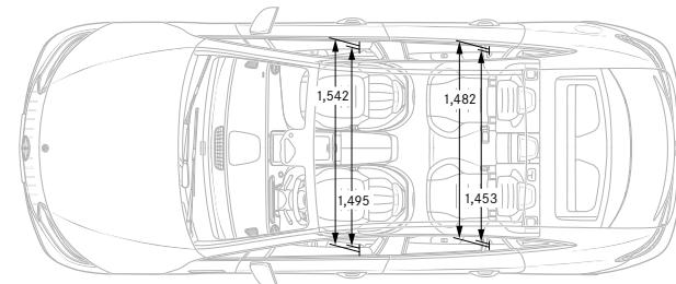
All measurements in millimetres. The dimensions shown are mean values and apply to standard-specification, unladen vehicles. Dimensions may vary slightly depending on the engine. Please consult your Mercedes-Benz Agent for further information
