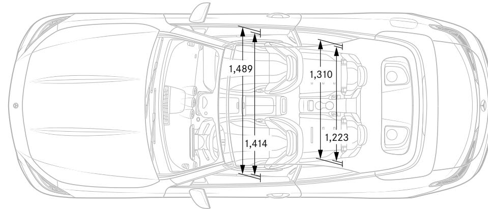
All measurements in millimetres. The dimensions shown are mean values and apply to standard-specification, unladen vehicles
