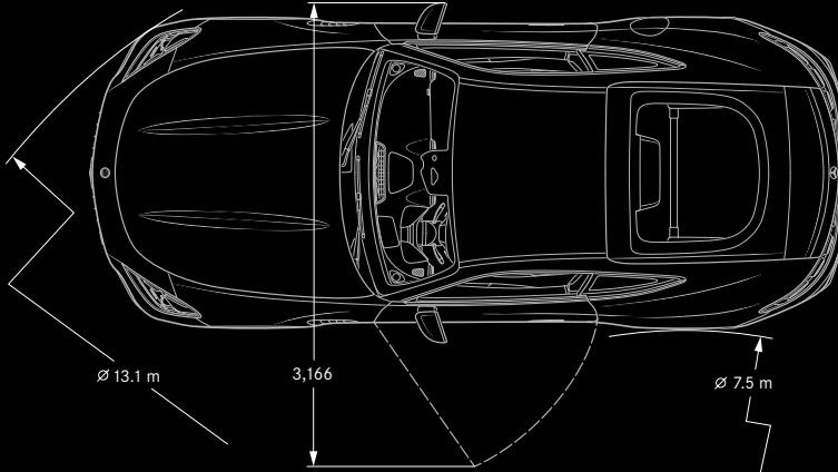
All measurements in millimetres. The dimensions shown are mean values and apply to standard-specification, unladen vehicles
