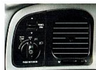
AUTOMATIC HEADLAMP ON/OFF DELAY. Headlamps automatically turn off after a selected interval to eliminate wear and increase security.
