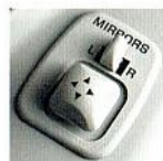
NEW HEATED DUAL POWER MIRRORS. Outside mirrors automatically defrost when the rear window defroster is turned on.
