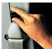
SEAT BELT HEIGHT ADJUSTER. For improved shoulder belt fit and comfort.
