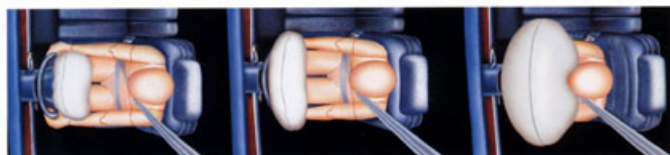
Shown here is an artist's depiction of a test of Grand Marquis' standard driver-side air bag Supplemental Restraint System. The air bag inflates during a moderate to severe frontal collision in less time than it takes to blink an eye.
