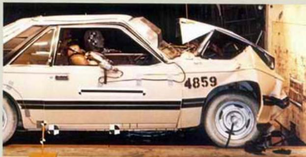
The doors on Capri feature strong, double-panel welded construction. Inside each door is a high-strength steel beam which enables each door to withstand a test load twice as great as Capri's curb weight.
