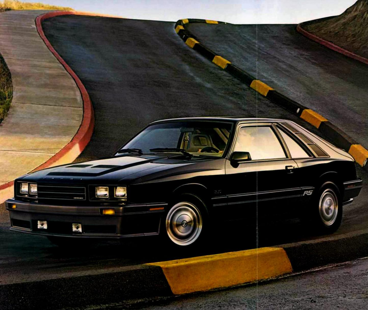
**C**apri RS gets its might from a standard 5.0-liter High-Output four-barrel V-8 engine with five-speed overdrive manual transmission. This small block V-8 cranks out an impressive 210 horsepower at 4800 rpm.\* If yellow-lines at 5200 rpm and red-lines at 5800 rpm. It's the stuff of which dreams are made.
