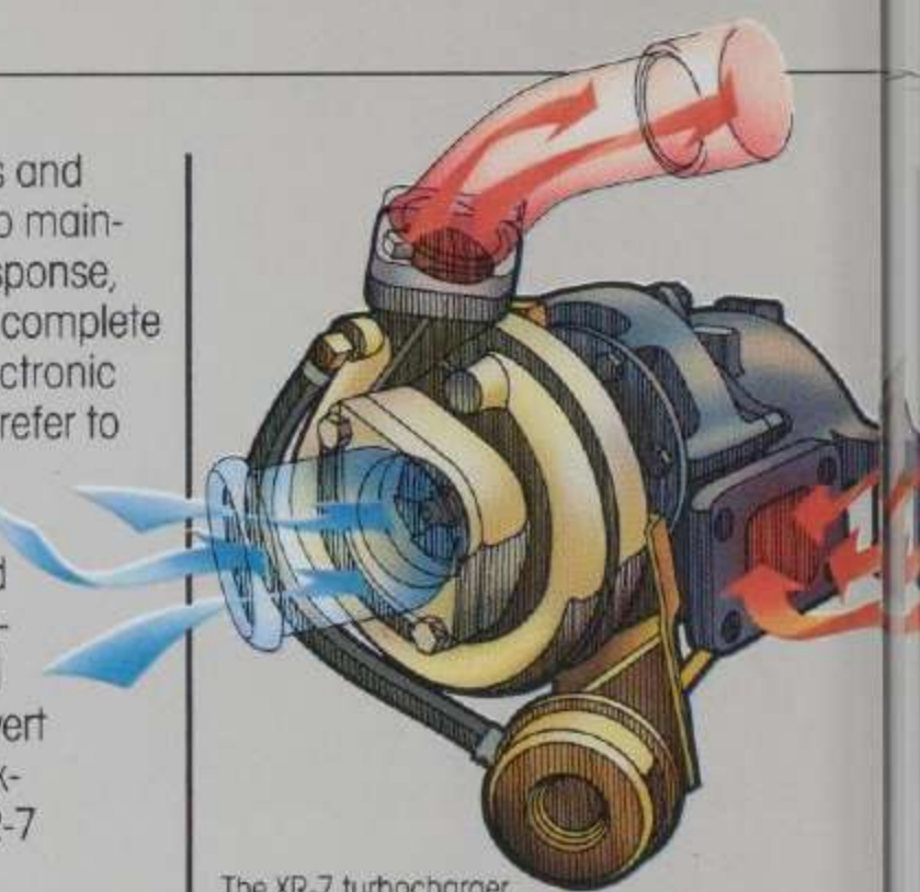
The XR-7 turbocharger boosts engine output under high-speed conditions.
