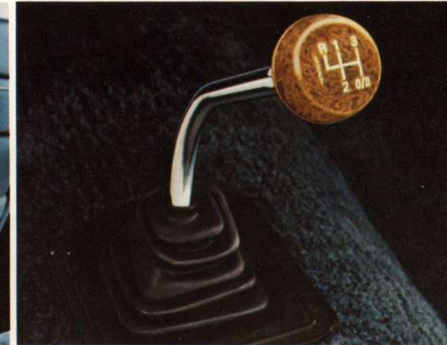
4-speed manual overdrive transmission
