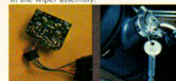
Solid-state ignition doesn't require breaker point replacement
