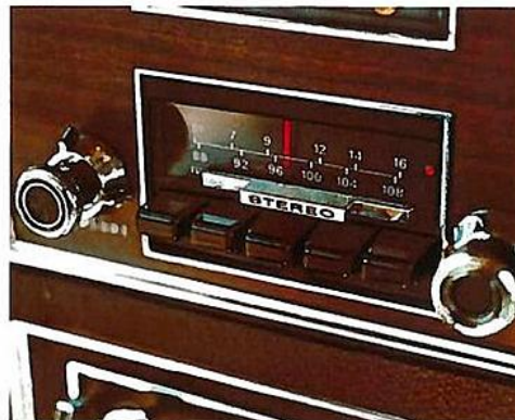
AM/FM/Multiplex Stereo Radio: Includes the features of the AM radio plus the choice of FM reception. Preselection of ten stations, five AM and five FM is available from five push buttons. With the use of the balance controls, an exact blending of sound may be achieved from the four speakers, one in each of the two front doors and two in the area below the rear window.
