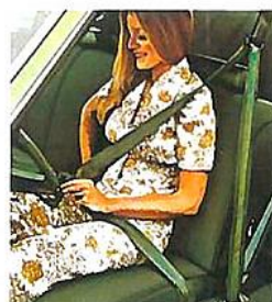
New 3 point restraint system allows you to lean forward comfortably to close the door, reach the instrument panel, etc., but it locks securely in place in the event of a sudden stop.
