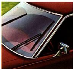
Articulated windshield wiper. In one clean sweep, it cleans a greater area.
