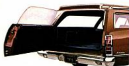
Our three-way tailgate. It swings open like a door for people and luggage with the window up or down... swings down flat for long loads.
