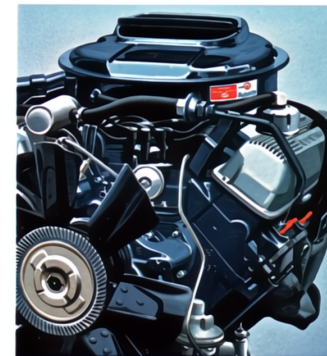
CJ 428 engine spews 335 horsepower with 440 lb. ft. of torque. 10.8:1 compression ratio. Huge 735 cfm capacity 4-barrel carburetor. Performance-tailored camshaft. Low-restriction air cleaner. Free-flow breathing characteristics.
