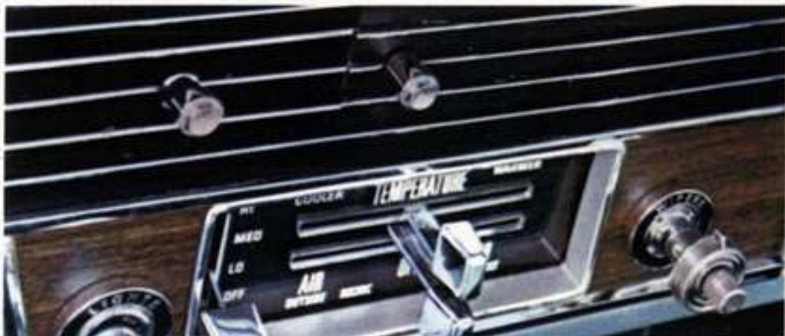
Deluxe Air Conditioner—cools, dehumidifies, filters out dust and pollen. A built-in instrument panel unit.
