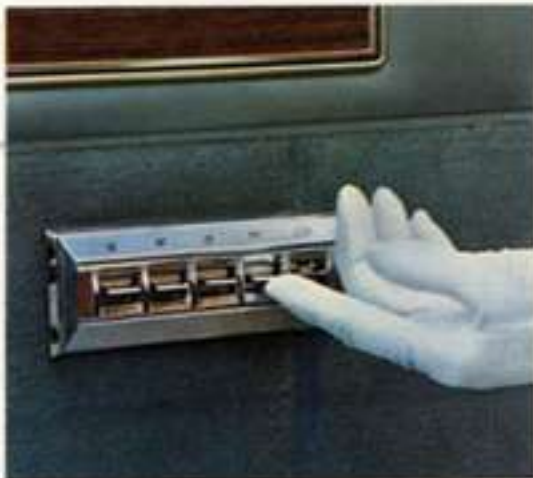
Power Windows—are a new item for '66. Beside the driver is a master control switch; an individual control is at each window.
