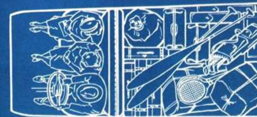
● With center and rear seats removed, the Station Wagon becomes an efficient utility hauling unit. Tail gate can be lowered and latched to increase loading length.
