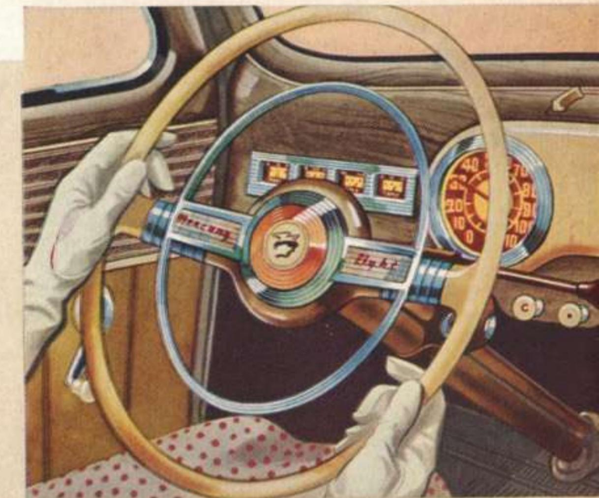
WITH MERCURY'S NEW Liquamatic Drive incorporating Automatic Gearshift you can keep *both* hands on the wheel in normal driving—go for hours without shifting gears!
