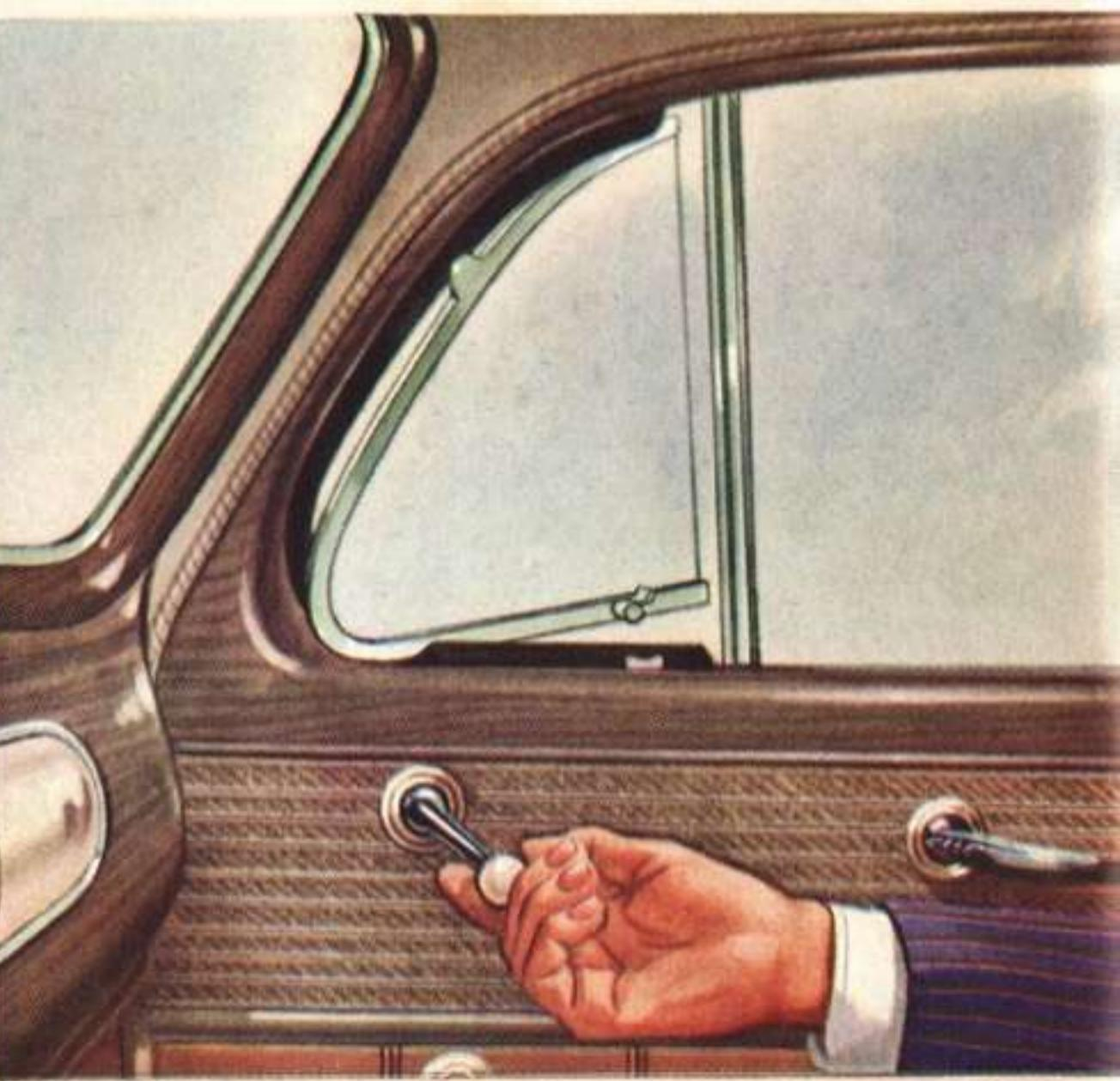
WING-TYPE quarter windows on Mercury closed bodies provide correct all-weather ventilation. There's no discomfort from drafts.
