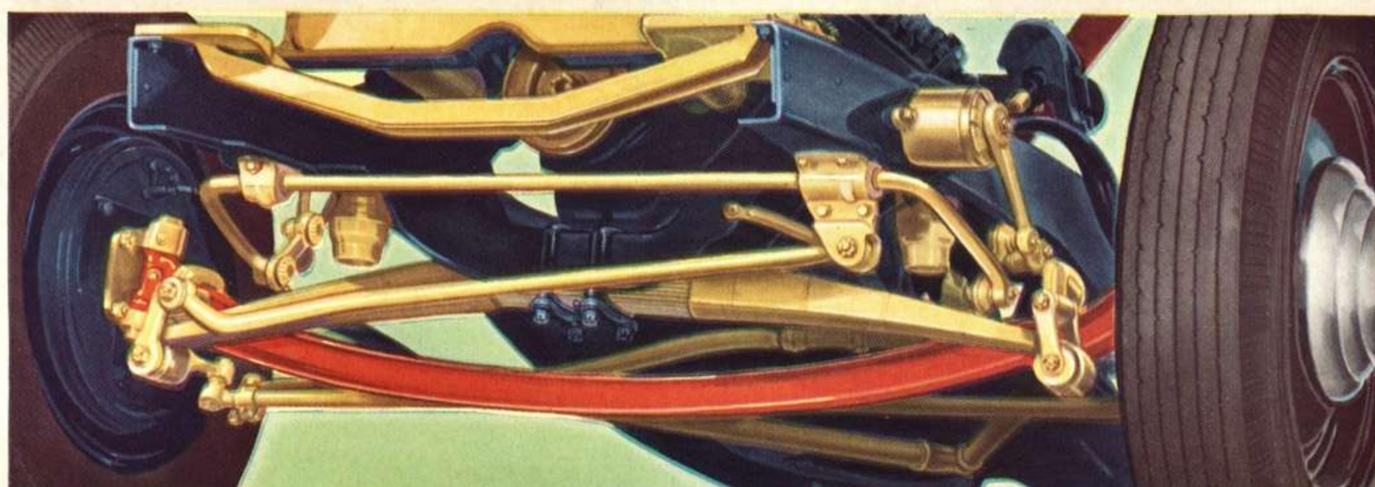
DOUBLE-ACTING hydraulic shock absorbers are of an improved design this year, for maximum riding comfort. Mercury springs, front and rear, are increased
