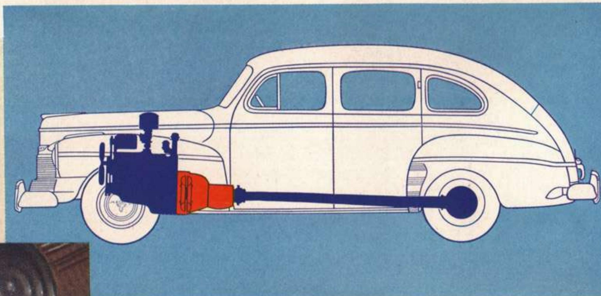
THE DIAGRAM above shows the engine, Liquamatic Drive and torque tube enclosing propeller shaft. Mercury Liquamatic Drive units are: Liquid Flywheel that transmits power from engine to transmission, and Automatic Gearshift which practically eliminates manual shifting.
