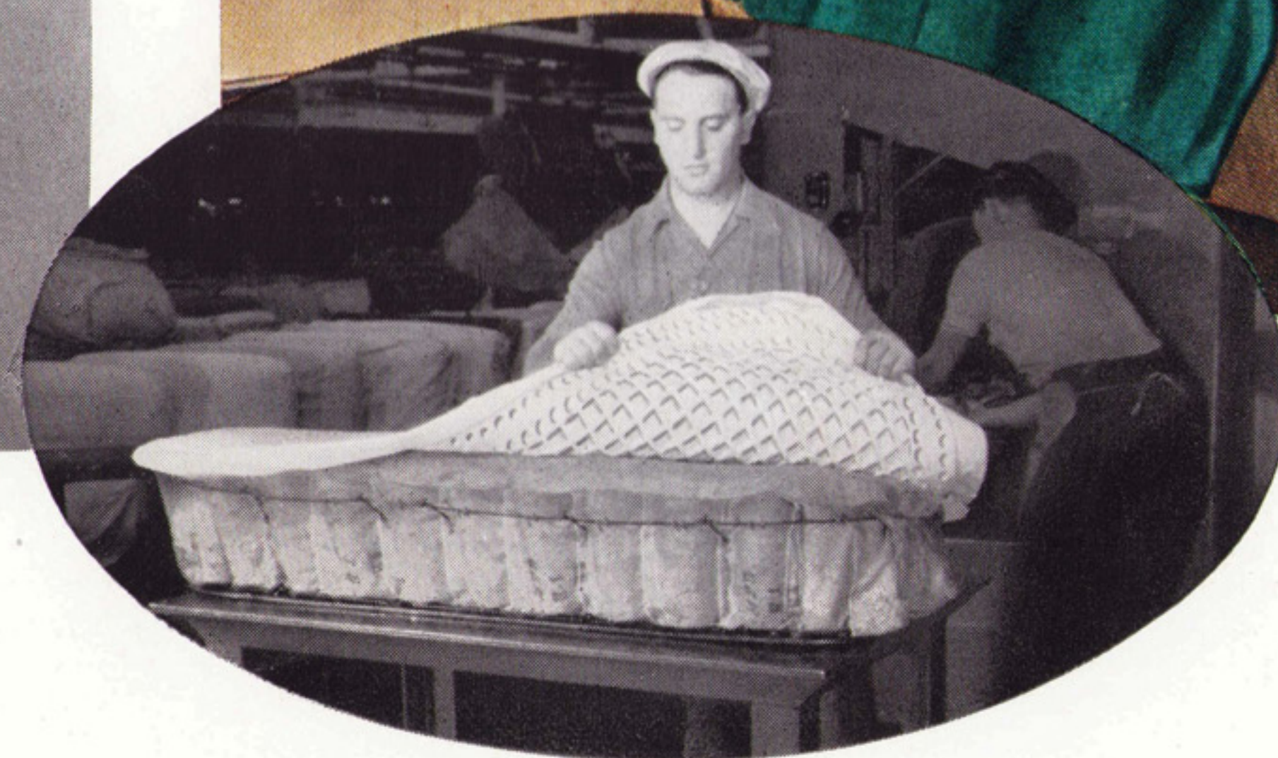
A NEW FEATURE of the famous Mercury ride: placing resilient foam rubber pads on flexible inner cushion springs.
