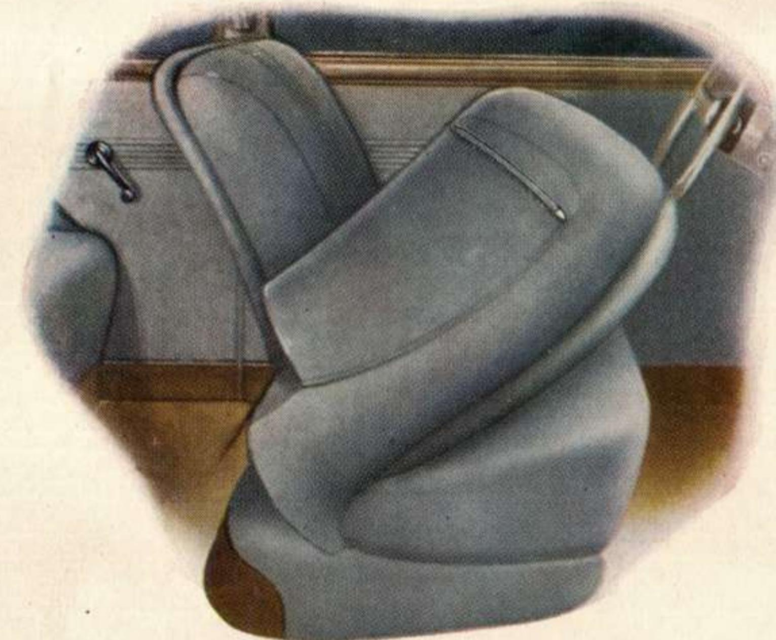
**For Easy Access** to the rear seat of all two-door types, each front seat back tilts inward, away from the wide door, as it swings forward. Every detail of the Mercury has been considered in the light of comfort and convenience.
