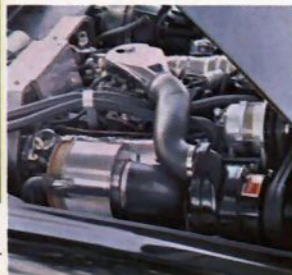
Paxton Supercharger. If you enjoy the thrill of exceptionally high performance, you get it with the optional Jet-Thrust V8 with Paxton supercharger. Gives you a 40 to 50% increase in reserve power as an extra margin of performance and safety for passing and highway cruising.
