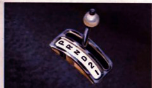
Avanti Power Shift. This unique transmission operates as an automatic, yet you can also shift up or down by hand, at will. Available only with the Avanti.
