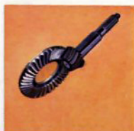
Six Axle Ratios. By accepting ring and pinion gears in various size combinations, the Lark differential permits maximum efficiency. One ratio, for example, is best suited to mountainous country. Others for flat country or for heavy traffic. You also can choose between a "fast pickup" ratio or one for best economy.
