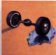
Twin Traction, Limited Slip Differential. In sand, mud, snow, ice or gravel, power is fed to the rear wheel that has the better grip. Thus you move off under slippery conditions which normally would call for chains or a tow. Available with all rear axle ratio combinations.
