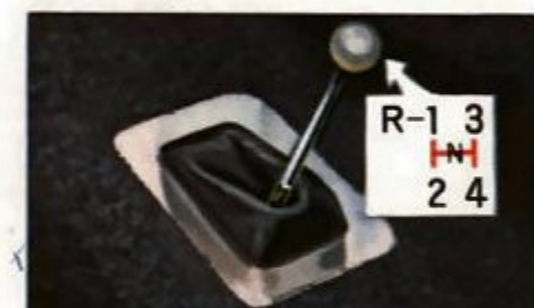
4-Speed Floor-Mounted Manual Shift for those who enjoy the full thrill of precision control. Available as an option on all Studebaker's V8 cars, the 4-speed stick shift, synchronized on all forward gears, lets you select the right gear for maximum efficiency or performance.
