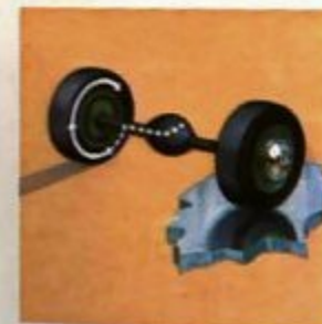
Twin Traction, Limited Slip Differential. In sand, mud, snow, ice or gravel, power is fed to the rear wheel that has the better grip. Thus you move off under slippery conditions which normally would call for chains or a tow. Available with all rear axle ratio combinations.
