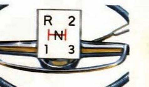
3-Speed Column-Mounted Manual. Because all gear teeth are cut at an angle, the standard manual transmission gives greater area of gear contact—smooth, easy, noiseless shifting and a high degree of durability. Available with and without overdrive.
