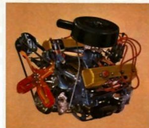
Thunderbolt 289 cu. in. V8 —High powered performance second only to the Jet-Thrust—yet remarkable economy on regular gasoline. Power Pack, with a 4-barrel carburetor and dual exhausts for even higher performance, optional on 289 and 259 V8's.
