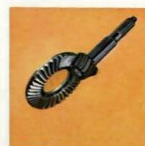
Twin Traction, Limited Slip Differential. In sand, mud, snow, ice or gravel, power is fed to the rear wheel that has the better grip. Thus you move off under slippery conditions which normally would call for chains or a tow. Available with all rear axle ratio combinations.
