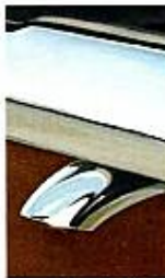
Chrome Exhaust Deflector —protects bumper from corrosive fumes.
