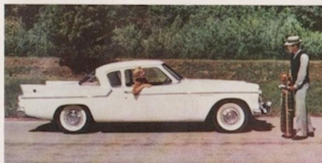
Brake fade is minimized with Studebaker's advantageous brake lining area-to-weight ratio. Large brake drums dissipate heat quickly, allow brakes to cool more rapidly for more efficient, safer stops.
