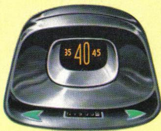
*A Safety Conscience . . .* is built right into your Scotsman. Studebaker's exclusive "Cyclops Eye" speedometer shows you your speed in magnified, illuminated numbers which change from green to amber at 35 mph., to red at 55 mph. A constant safety reminder.
