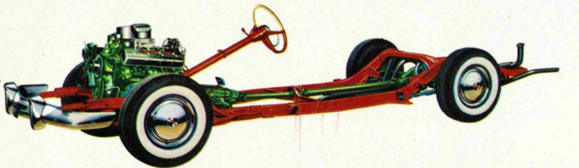
Studebaker Station Wagon Pyramid Design frames have five crossmembers, giving greater rigidity and safety, lower center of gravity. Double-flanged box-section construction, and electrically welded steel body panels give added strength and protection to entire passenger compartment; minimize rattles, squeaks.
