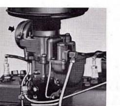
Exclusive automatic choke! Full automatic carburetor heat control, octane selector and automatic spark control. Fast starting, freedom from "ping" and every ounce of power developed by the fuel put to useful work!
