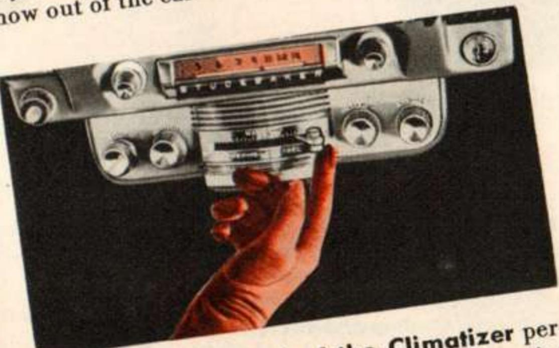
The Thermo-control of the Climatizer permits simple, quick regulation of the heating system. You can set it for the desired temperature range by moving the central lever to the right or left. Knobs on either side control the circulating fan and the defroster.
