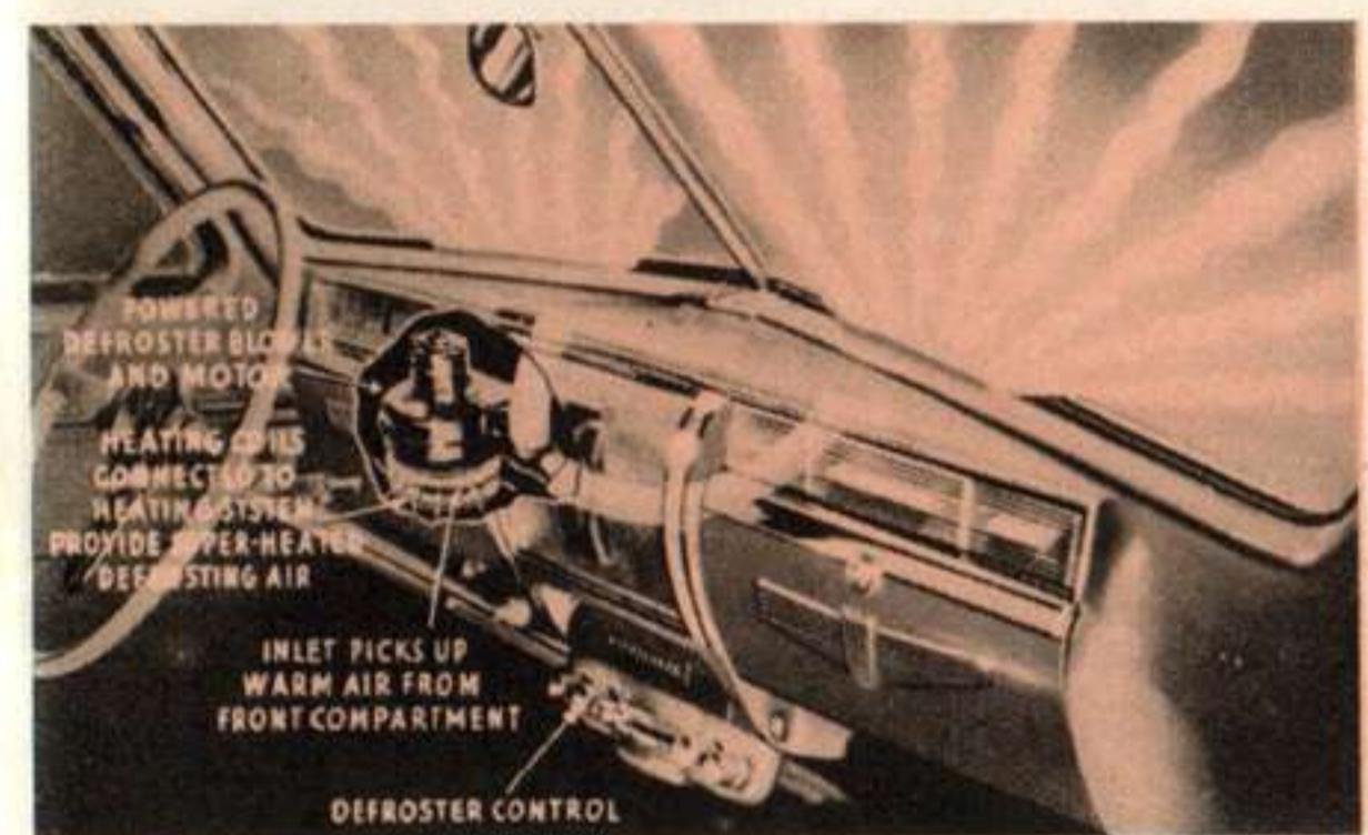
**The Climatizer Defroster** has a powerful blower with extra heating coils. 50 cubic feet of heated air per minute is discharged over the windshield—ample defrosting power for clear, safe vision under all driving conditions.
