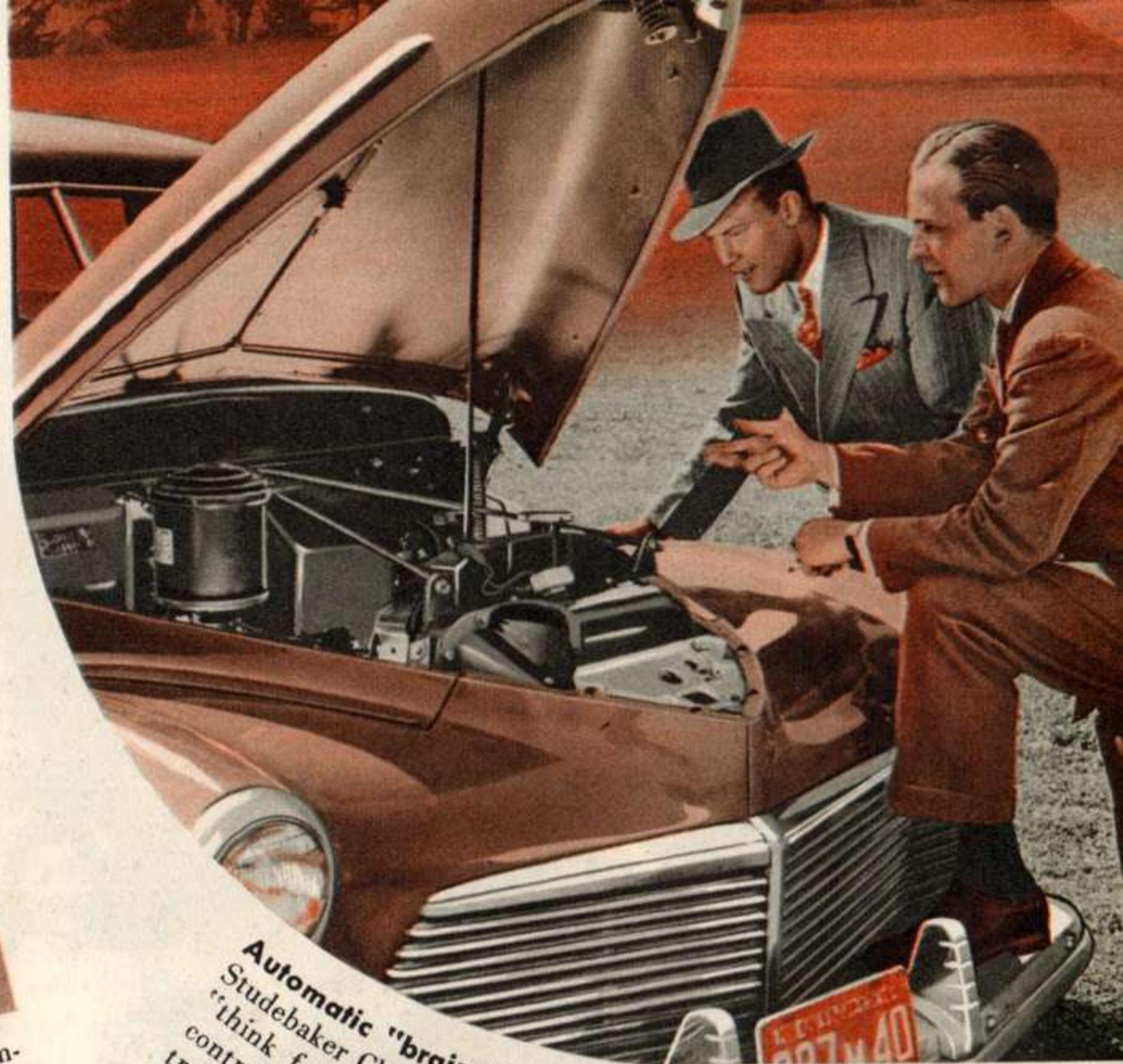
Automatic "brains" remember so that you can forget. Studebaker Champion performance is assured by engines that "think for themselves" with automatic choke control, spark control, water temperature thermostat and thermostat for controlling manifold heat. The carburetor provides the exact mixture of gasoline and air either for maximum performance or economy.
