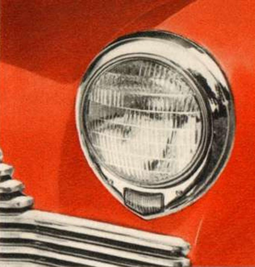
The sealed beam headlights of the 1942 Studebaker Champion are faired into the fender as smoothly as the landing lights on a Stratoliner.
