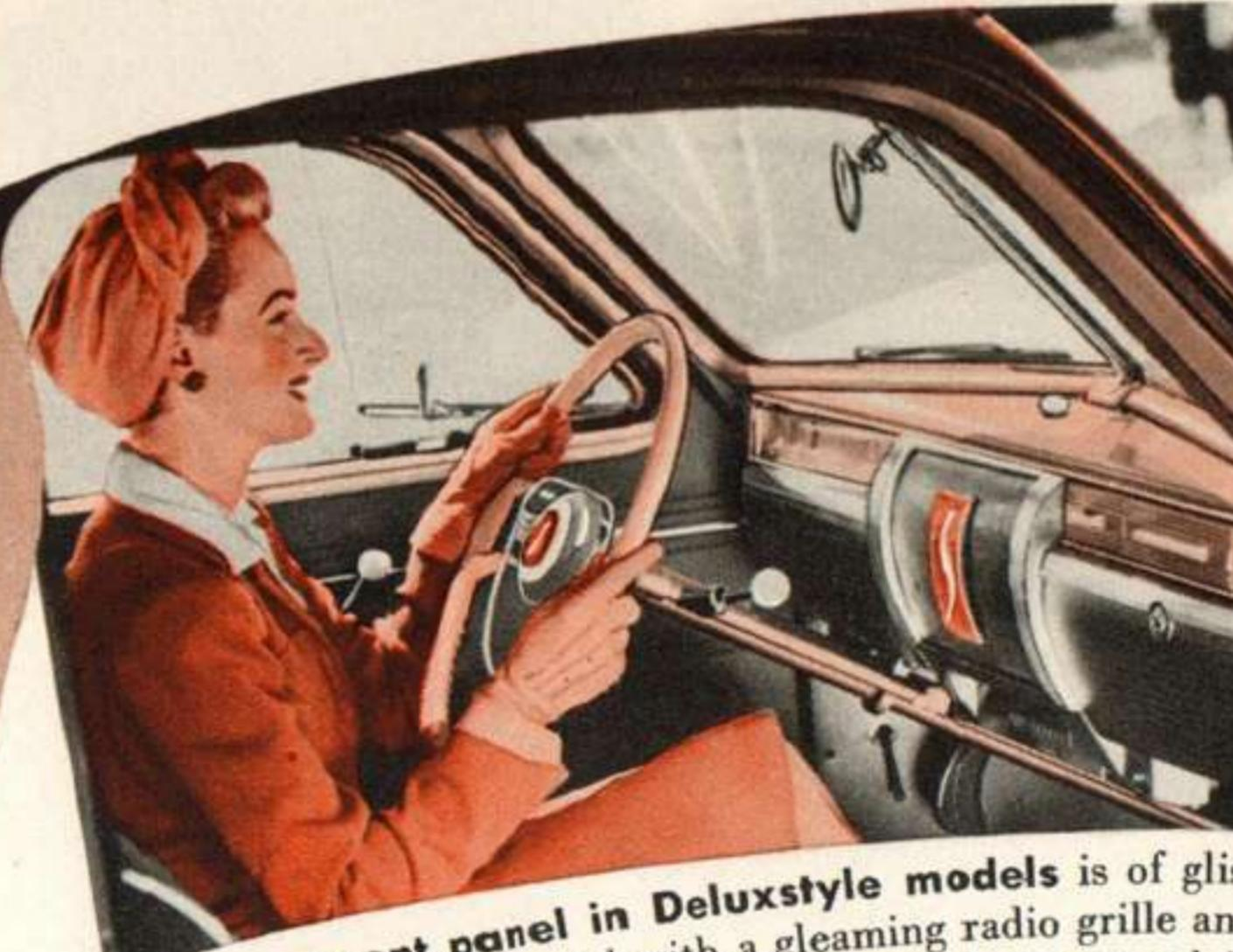
The instrument panel in Deluxstyle models is of glistening engine-turned steel with a gleaming radio grille and plastic control buttons. Instrument board is lacquered in two-tone color combination to harmonize with upholstery in Custom models. Gearshift lever is on steering column.
