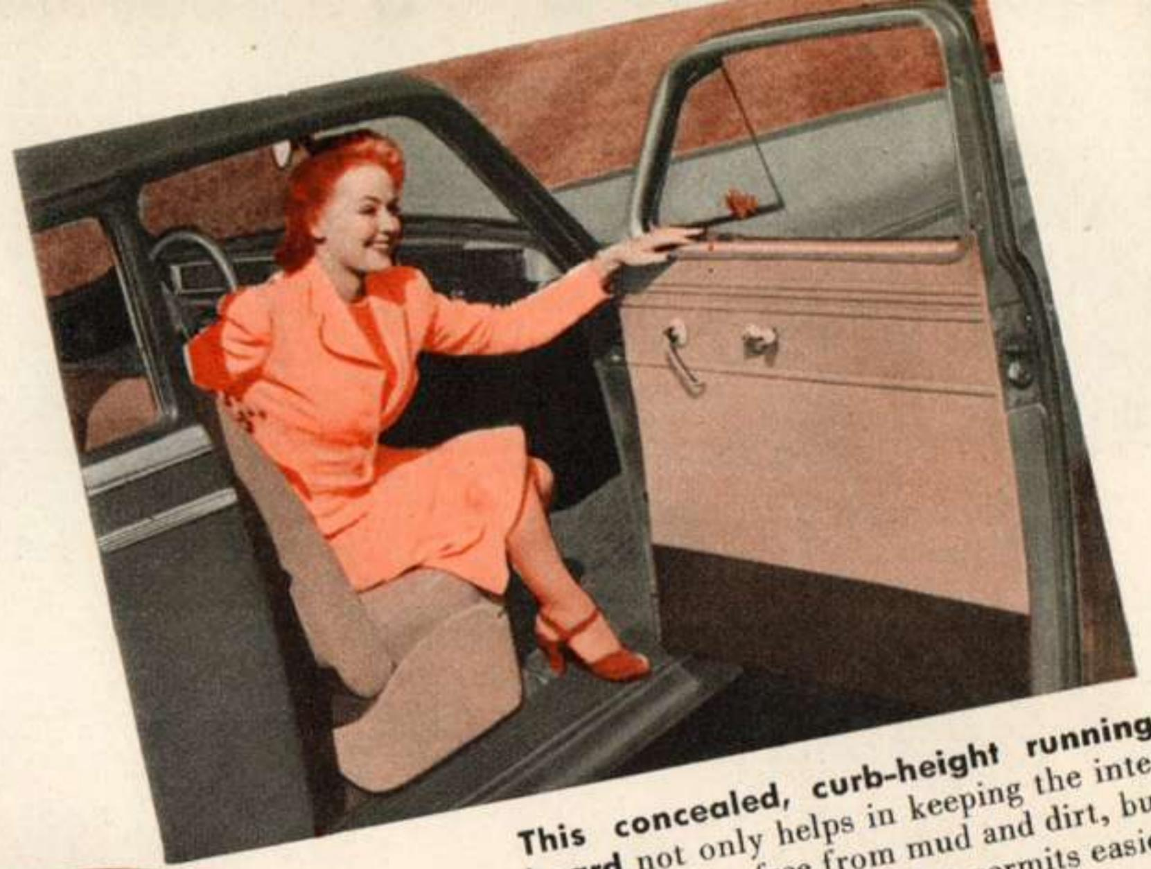
This concealed, curb-height running board not only helps in keeping the interior of the car free from mud and dirt, but it is also a safety factor that permits easier ingress and exit for passengers.
