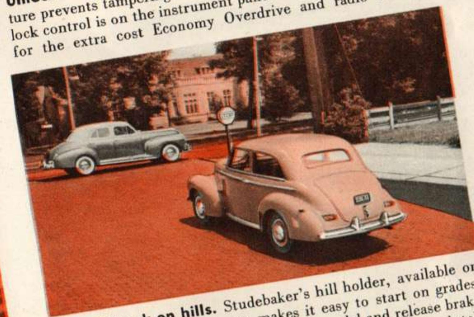
**No roll-back on hills.** Studebaker's hill holder, available on the Champion at extra cost, makes it easy to start on grades. Just brake to a stop, step on the clutch pedal and release brake. The hill holder keeps you there until you again engage the clutch.
