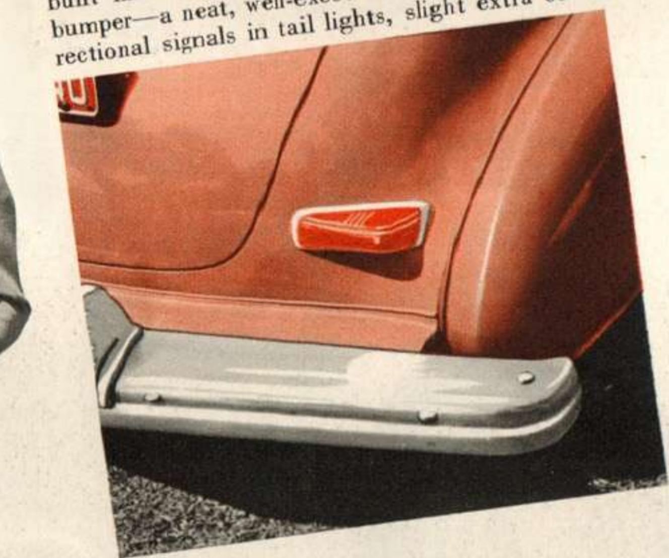
The **after deck of the 1942 Champion** is in perfect harmony with the low-swung front end. The rear fenders are faired smoothly into the body. The bumper is exceptionally massive and rugged in design. The accurately fitted trunk lid, plus sponge rubber seal, makes trunk dustproof and weather-tight.
