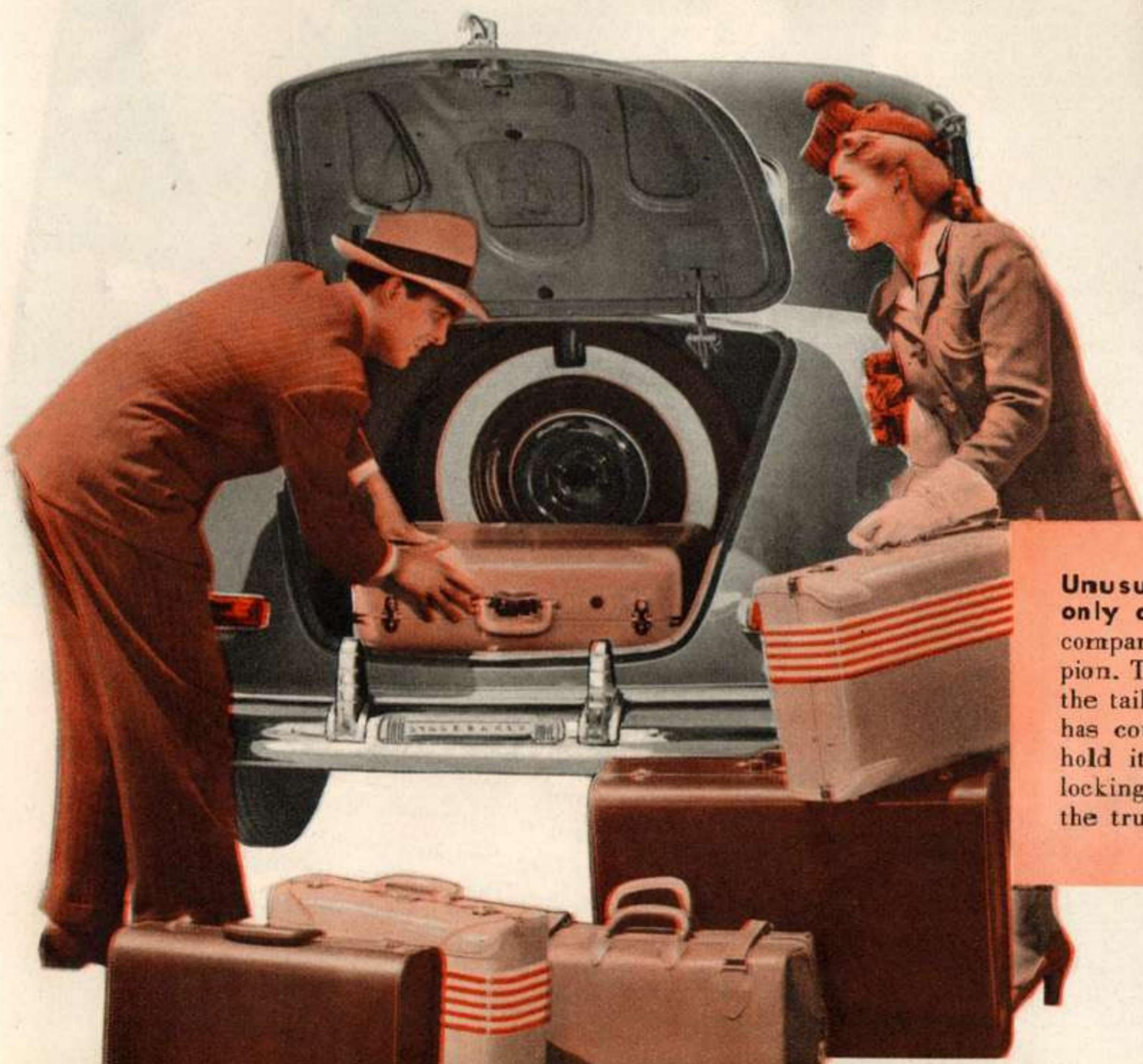
Unusual roominess isn't the only advantage of the trunk compartment of the 1942 Champion. Trunk interior is lighted by the tail lamps; the lid on Sedans has counterbalanced hinges that hold it open or closed without locking. Rubber moulding seals the trunk against rain and dust.
