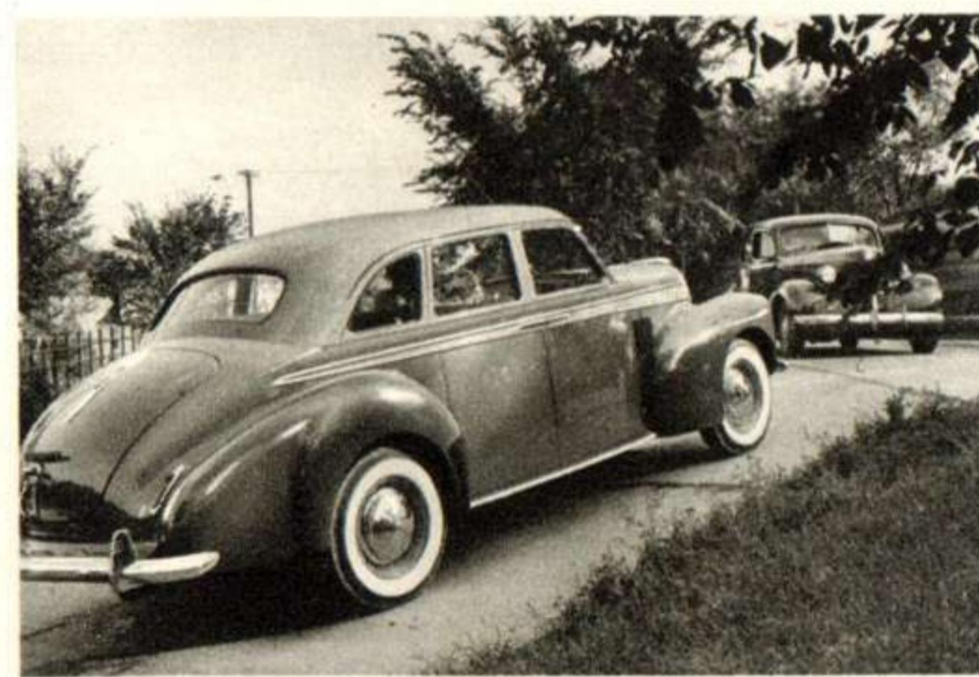
You don't roll back when you stop on an upgrade—That's because Studebaker's automatic hill holder keeps your Commander or President securely stopped until you're ready to go. You just hold the clutch pedal down and you can safely release your brake pedal.
