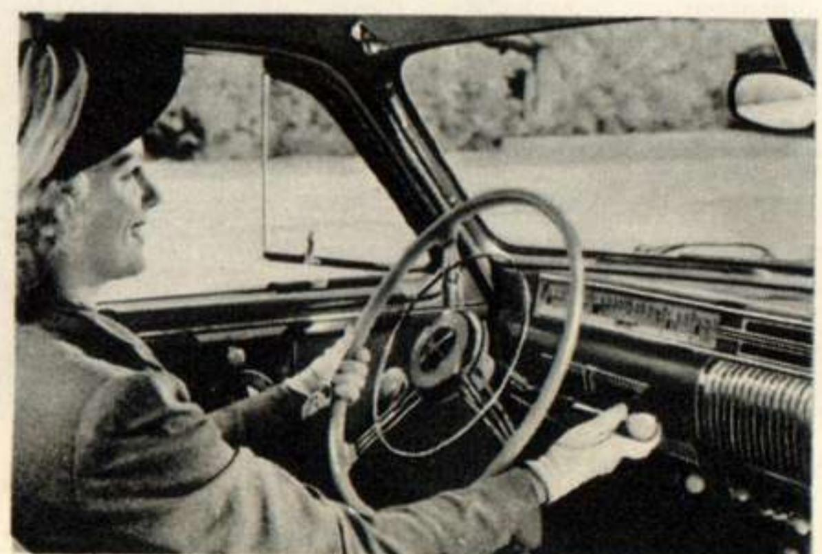
**You shift gears with finger-tip ease in a Studebaker**—The gearshift lever is conveniently located immediately below the steering wheel. All the driving controls are easily accessible.
