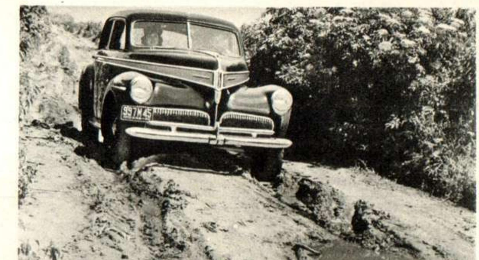
**Rough spots like this seem smooth** thanks to Studebaker's exclusive planar independent suspension and finest hydraulic shock absorbers. Studebaker's front wheel suspension is self-stabilizing. You experience none of the sidesway of coil spring cars with Studebaker's big transverse spring.
