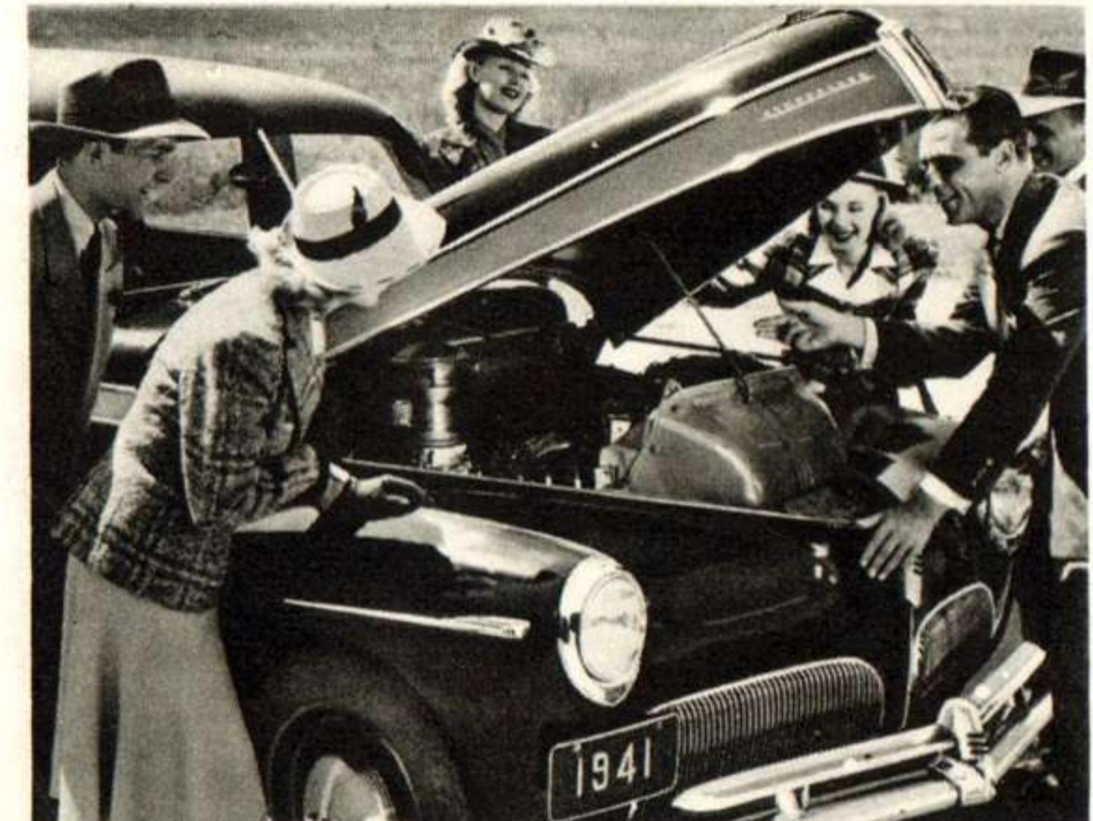
**Almost everything is automatic in these Studebakers**—They have automatic choke control, automatic spark control, automatic water temperature thermostat, and a thermostatic "brain" to control manifold heat. "Tailor-made" carburetors mix gasoline and air "just right."
