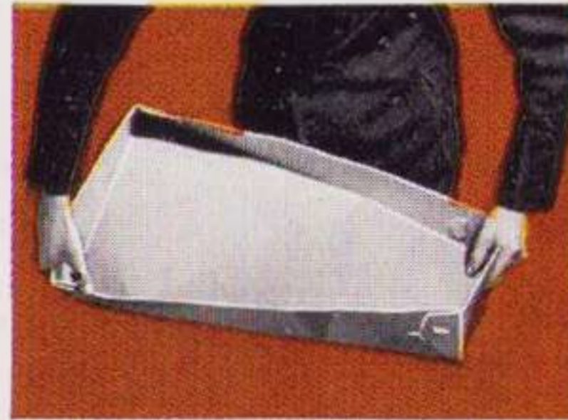
Look how easy it is to crush and twist the three-sided "U" box pictured above. That's the type of reinforcing used in most cars.
