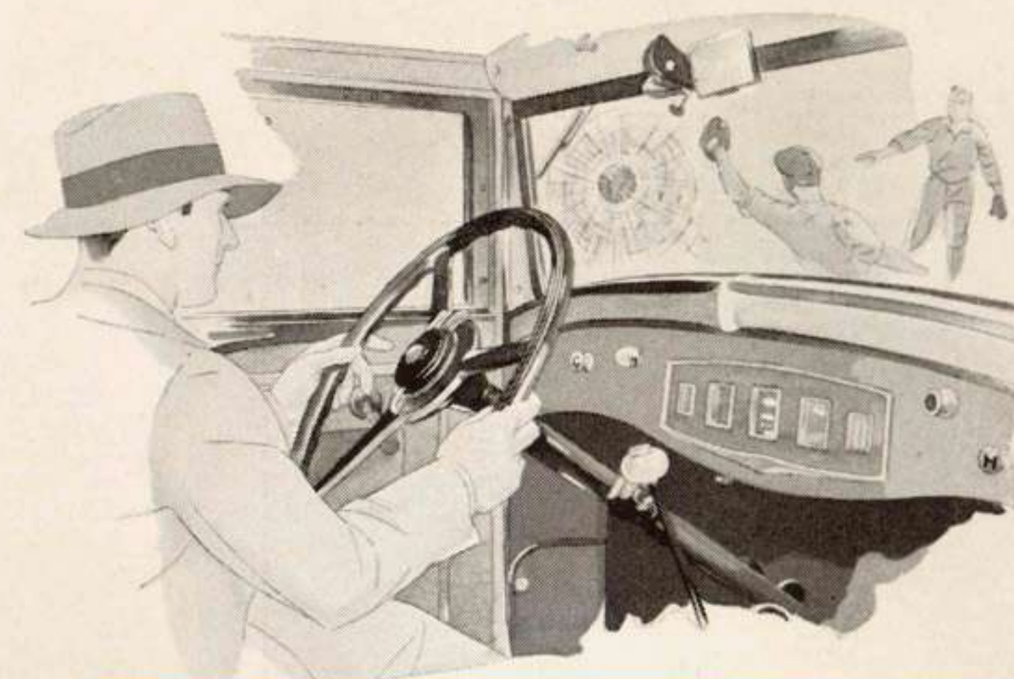
(LEFT) Safety glass in windshields of all models offers an added measure of protection in Commander Eight bodies. In Regal models safety glass is used in side and rear windows as well.
