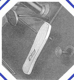
(ABOVE) New rubber treadle foot accelerator relieves strain on long drives—stays cool—protects dainty slippers.
