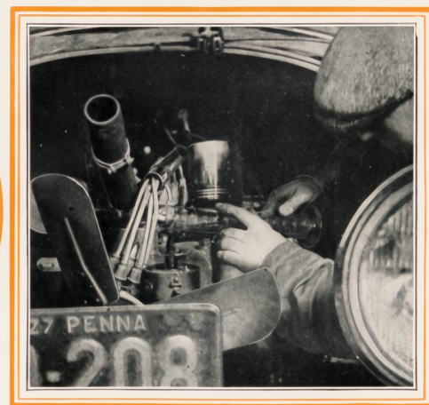
Nothing was left to doubt. Here you see an official of the American Automobile Association checking compression ratio on Commander model selected at random from dealers' stock—to compare with 25,000-mile Commanders
