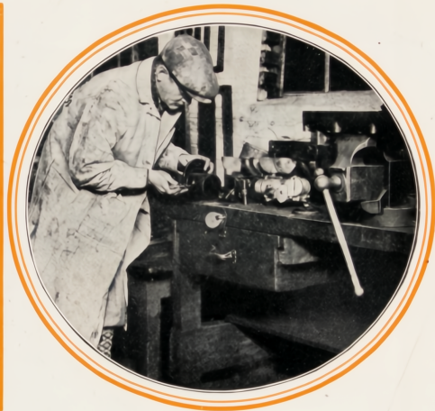
American Automobile Association engineer checking Studebaker piston. The three 25,000-mile Commanders were disassembled and checked meticulously to make certain these record-breaking cars were strictly stock models
