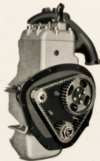
The timing gears are driven by silent chain; lubricated by oil pumped from crankcase; accessible outside adjustment.
