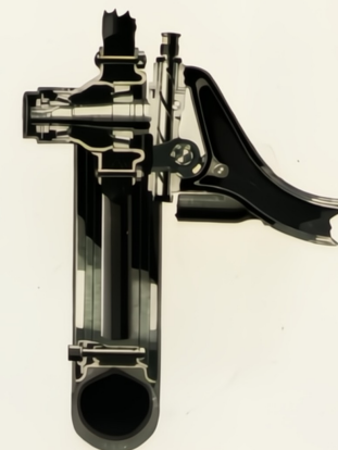
Steering knuckles, steering arm, etc., are alloy steel drop forgings, heat-treated to provide factors of safety for the shocks to which they may be subjected.
