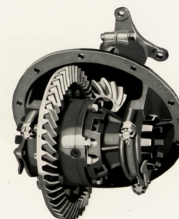
The rear axle pinion carrier may be removed without taking the axle from the car. Gears are drop forged chrome nickel steel.
