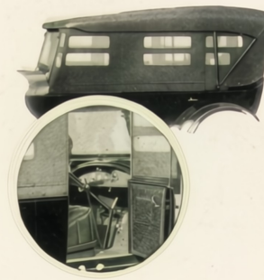
Storm curtains which open with the doors are bound on three sides by steel rods to insure proper protection from weather.
