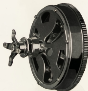
The single plate dry disc clutch makes gear shifting quiet and easy. Clutch brake serves to prevent spinning of transmission gears after clutch is disengaged.
