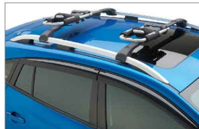
J-style carrier folds down when not in use.
