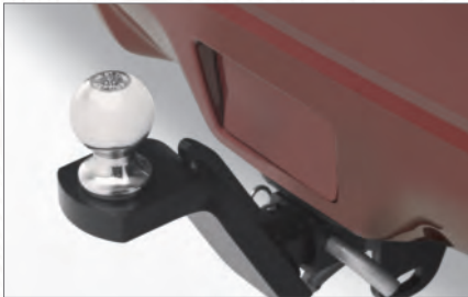
Trailer Hitch. Rated at 200 lbs tongue weight with 1,500 lbs of towing capacity. Engineered to the same rigorous standards as the rest of the XV Crosstrek. Hitch ball not included. Trailer brakes may be required. Excludes Hybrid models.
