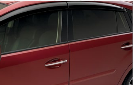
Side Window Deflectors. Designed to let the fresh air in while helping to keep the rain out of the vehicle. Black acrylic plastic construction is designed specifically for an exact fit on the Impreza models. May not be legal in all states. Please check the laws of your state.
