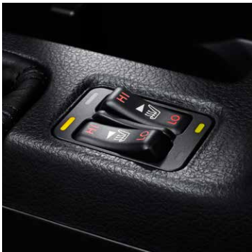
Front Seat Heaters* 3 Available heated front seats offer two settings, for rapid heating or soothing warmth.
