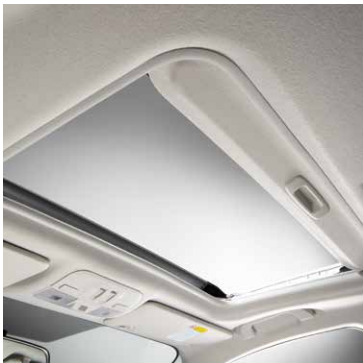
Power Glass Sunroof* 1 This available sliding sunroof with manual sunshade is tilt-adjustable and delivers a wide panoramic view and fresh breezes for front and rear passengers.
