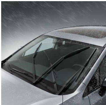
Automatic Rain Sensing Windshield Wipers* 2 Available automatic windshield wipers detect rainfall on the glass and adjust their wiping intervals and speed accordingly.
