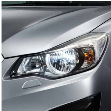
HID Headlamps with Auto Levelizer* 1 Available high-intensity discharge headlamps provide illumination that's more like daylight. The auto-levelizer helps to ensure that the headlamps are always pointed at the correct angle for the best visibility.
