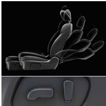
8-way Power Adjustable Driver's Seat* 1 Available for driver's seat, this allows you to quickly find a comfortable and confident seating position by 8-way power adjustment.
