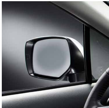
Heated Door Mirrors* 3 Featuring a design that's large to improve your visibility, but also shaped to reduce wind noise, include electric heating.
