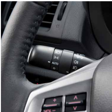
Auto On/Off Headlamps* 2 A light sensor turns on the headlamps automatically at dusk, and shuts them off when you remove the key from the ignition.
