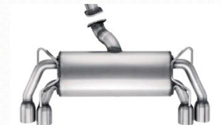
**SPT Performance Exhaust System.** These exhaust systems feature full stainless steel construction with smooth mandrel bends for low restriction and that famous boxer engine sound. WRX STI system shown. Available for WRX 4-door and 5-door.
