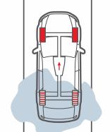
Matched to the 4-speed automatic, the Active AWD system monitors parameters such as wheel slippage and vehicle speed, actively adjusting power to the front or rear wheels for optimal adhesion.
