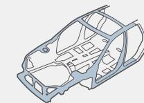
Engineered for exceptional strength to help maintain the integrity of the cabin structure, the innovative Subaru ring-shaped reinforcements around the passenger compartment also help dissipate crash-impact energy away from occupants.
