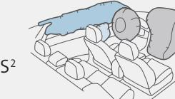
An intelligent front air bag system senses front-passenger seat occupancy to determine the safest deployment level. Side curtain air bags help protect front and outboard rear seat passengers.
