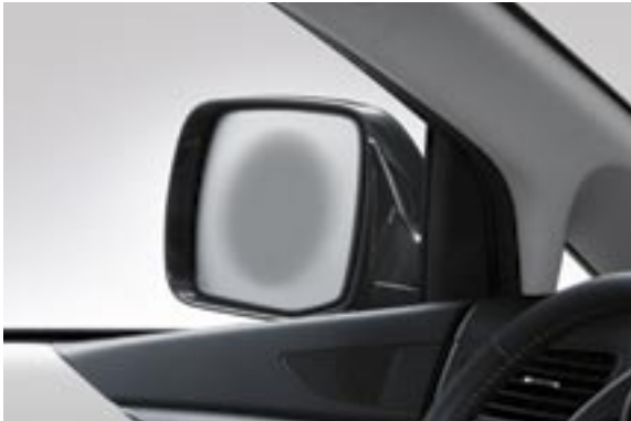
Heated door mirrors The built-in heater evaporates fog, drips and snow clear of the mirror surface. Very useful on wet or cold winter days.
