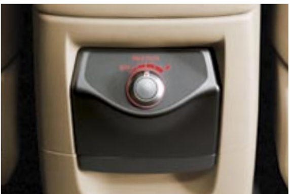
Individual rear cooling system (Limited 5+2 passengers) When the air conditioning is on, the overhead air-vent blows cooled air to the rear compartment, including the second row. That way, everyone can enjoy the cooling effect.
