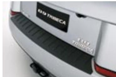
Cargo step panel Rugged plastic resin cover helps protect upper surface of rear bumper.
