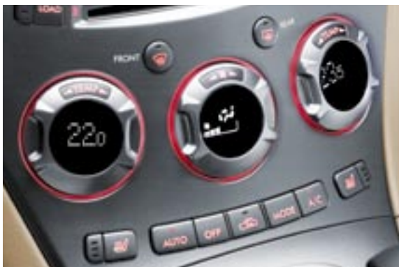
Dual-zone air-conditioning system The air-conditioning system is separated in two zones, one for driver’s side and the other for the front passenger’s side. So, the temperature for both driver and front passenger can be individually regulated for comfort.
