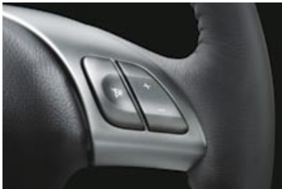
Audio satellite switches An audio remote control switch is installed on the steering wheel, so you can safely adjust and control the audio system as you drive.
