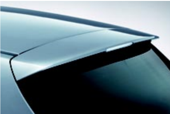
Roof spoiler While it adds to the B9 Tribeca’s sporty looks, this is also a carefully engineered addition to the goal of improved aerodynamics.
