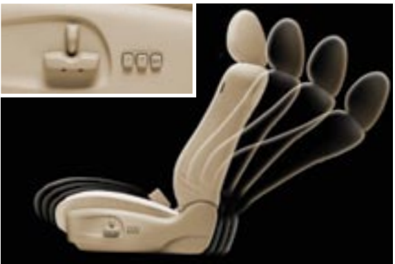
Power front seats The 8-way power-adjustable driver’s seat and 4-way power front passenger seats are both manually adjustable for correct lumbar support. The leather front seats of Limited models have 3-stage seat heater function, and its driver’s seat also incorporates a memory function for two different drivers’ settings.
