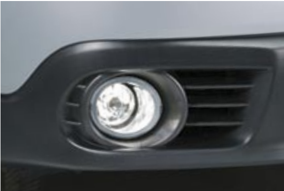
Front fog lamps Fog lamps light up a wide area of road surface in fog, snow or other bad weather to improve your vision for safety's sake. They work together with the front low-beam headlamps to give a fuller view of the road ahead.
