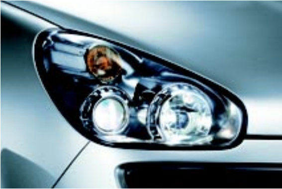
Headlamps (3-cylinder shape) By separating out the individual features of projector type low-beam, multi-reflector high beam, and turn indicator, the 3-cylinder, 3-D construction is both stylish and practical.
