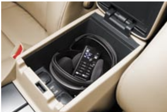
Centre console box The cover has a tray for small items and a drawer behind with access to another compartment. An auxiliary audio input jack and two sets of 12-volt power outlets are also incorporated.
