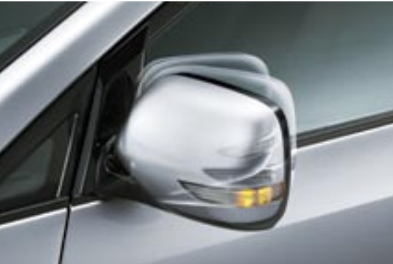
Power-folding door mirrors The door mirrors are obviously aerodynamic in their design with a dirt repellent shape. These mirrors are also power-folding for trouble-free narrow space parking. The built-in turn signal uses LED for extra visibility.
