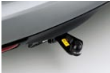
Trailer hitch Maximum towing capacity 2,000 kg.
