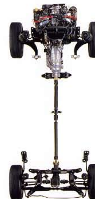
Powertrain components are laid out in a straight line and close to the chassis' centerline, giving agility while providing greater stability.
