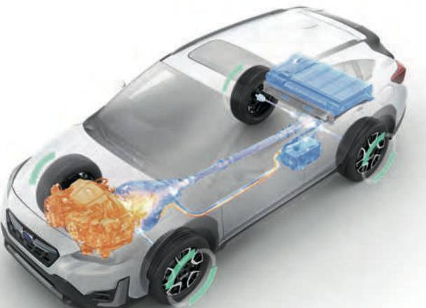
In **everyday driving**, the system will run on a combination of electric and gas power. It can also recover energy via regenerative braking.
