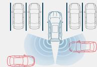
**Rear Cross-Traffic Alert**<sup>15</sup> alerts you with an audible warning and a flashing indicator on your exterior mirror and Rear-Vision Camera display if it senses traffic approaching from the side as you are backing up.
