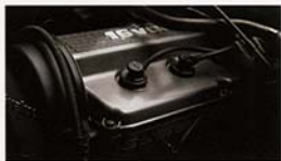
The 2-door JX Sidekick's new 1.6-liter, 4-cylinder, SOHC engine delivers 95 hp at 5600 rpm, along with one of the best EPA estimates in the 2-door SUV class: 23 mpg city, 26 mpg highway, with its 5-speed manual transmission. A 3-speed automatic transmission is also available.
