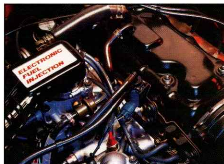
1.3 litre, electronically fuel-injected, single overhead cam engine.
