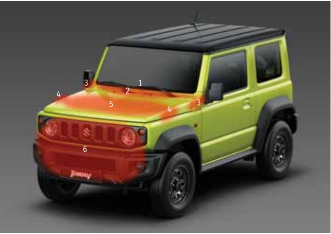
Injury mitigation body for pedestrian safety In the unfortunate event of a collision with a pedestrian, head and leg injuries are mitigated by a bonnet and surrounding parts that are designed to absorb impact.
