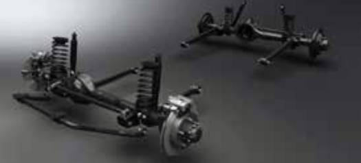
3-link rigid axle suspension with coil spring Settle for nothing less than full-width rigid axles in both the front and rear, which help the Jimny ensure superior grip on diverse surfaces. When an obstacle pushes one wheel up, the axle presses the other wheel down to increase tyre contact in rough road conditions.
