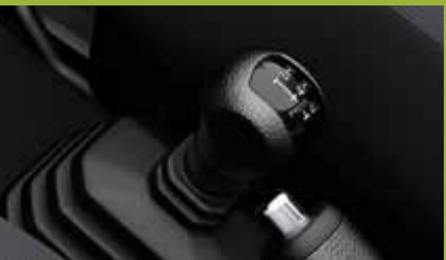
4WD with low range transfer gear At your command, the Jimny adapts to every situation. Shift the transfer lever to the 4L mode when the going gets tough for maximum torque and traction. On flat off-road trails and snow-covered roads, enter 4H to enjoy 4WD traction at higher speeds. Once you return to paved roads, shift to the 2H (2WD) mode for a smoother, quieter and more fuel efficient ride. Let ALLGRIP PRO satisfy your adventurous mind with its on and off-road mastery.
