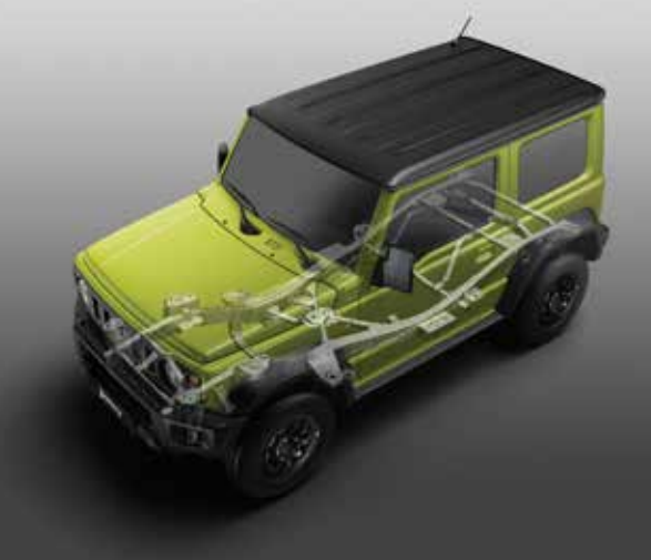
Rigid ladder frame From the very first generation, the Jimny has always featured a ladder frame that offers a solid foundation for serious off-road performance.
