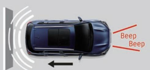
**Rear parking sensors** (Turbo Prestige only): Ultrasonic sensors in the rear bumper help with parking by detecting obstacles and issuing warnings that the driver can see on the multi-information display and hear as beeps.
