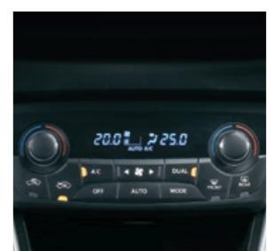
**Dual-zone automatic air conditioner:** The air conditioner gives personalised comfort by letting the driver and front passenger set temperatures independently of each other.
