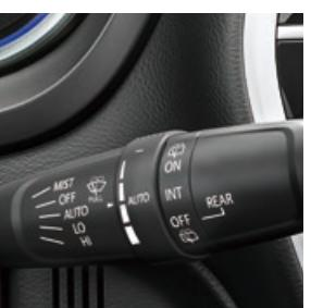
**Automatic wipers and lights** (Turbo Prestige only): The wipers start automatically when they sense raindrops, adjusting their speed to match the extent of rainfall and the speed of the car. Head and tail lamps turn on and off in accordance with the ambient brightness.
