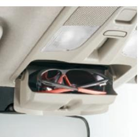
**Overhead console with map lamps:** The overhead console incorporates map lamps and a holder for sunglasses.
