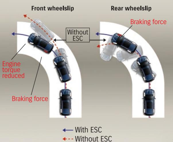
**ESC (Electronic Stability Control):** If the wheels lose traction, ESC automatically adjusts the engine and brakes to help keep the driver in control.
