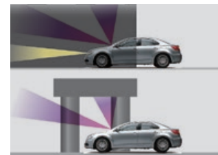
Auto headlight system Turns lights on and off to suit driving conditions
