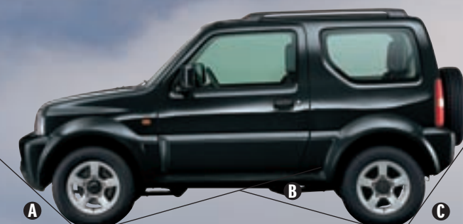
A 37° Approach angle (default setting, unloaded Jimny) B 31° Ramp breakover angle C 46° Departure angle
