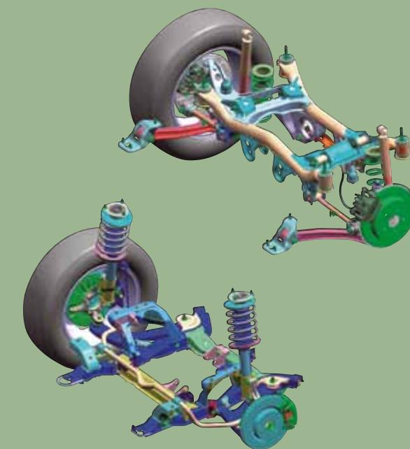
Agility and sporty handling is delivered through the independent suspension featuring front MacPherson struts and rear multi-link geometry. Both work in tandem to increase on-road responsiveness and off-road handling.
