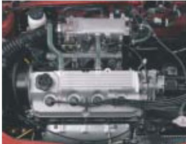
16x4 All-Aluminium Hypertech Engine
