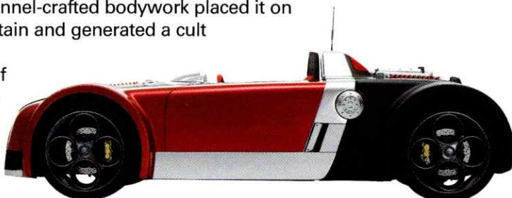
adjustable suspension and detachable, lightweight, recycled-plastic body panels for easy customizing. For the interior, designers chose light and supportive bucket seats for agility and comfort, as well as storage space behind the seats for helmets. As an added perk, the vehicle has a Wrist Mount System — sponsored by Seiko Instruments Inc. — that serves as a door-lock release, driver identification, wireless communication tool and hands-free mobile phone.
