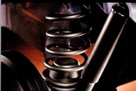
MacPherson Strut Suspension
